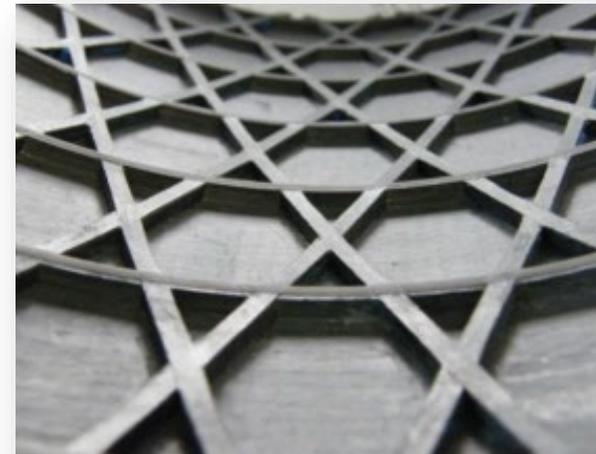
COMPOSITE ANISOGRID CONCEPT MADE OF UNIDIRECTIONAL RIBS
