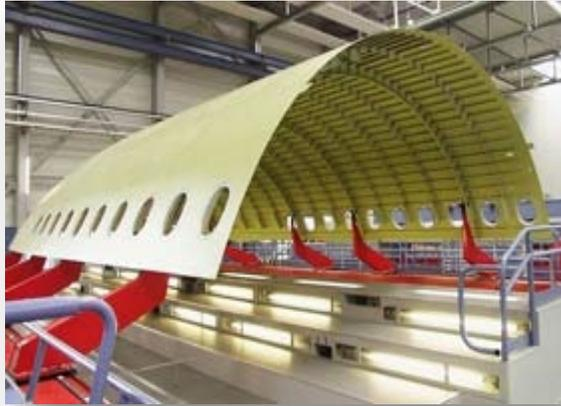
A BASIC LOAD-CARRYING SHELL REINFORCED BY FRAMES AND LONGERONS IN THE BODIES, AND A SKIN-STRINGER CONSTRUCTION SUPPORTED BY SPARS AND RIBS IN THE SURFACES
