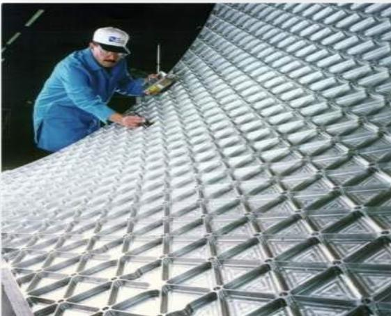
AN ISOGRID IS A TYPE OF PARTIALLY HOLLOWED-OUT STRUCTURE FORMED USUALLY FROM A SINGLE METAL PLATE (OR FACE SHEET) WITH TRIANGULAR INTEGRAL STIFFENING RIBS (OFTEN CALLED STRINGERS)
